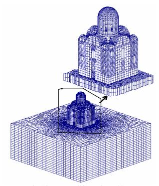
Fig. 5 Structure - soil interaction problem
