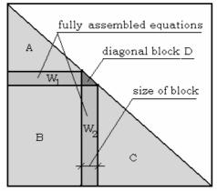
Fig. 2. Block factoring of stiffness matrix
