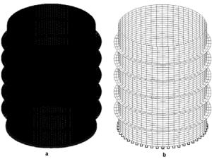
Fig. 4. Ribbed shell with discrete welded connection. a – computational model with fine mesh, b –model with a coarse mesh
