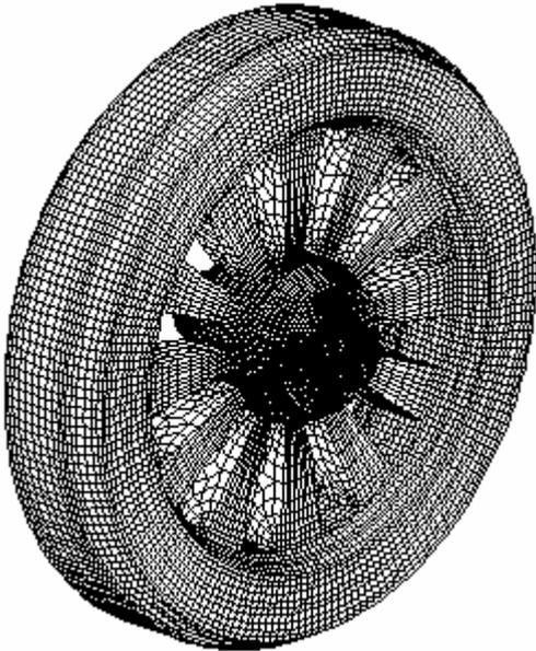
Fig.3 A finite element model of a wheel
