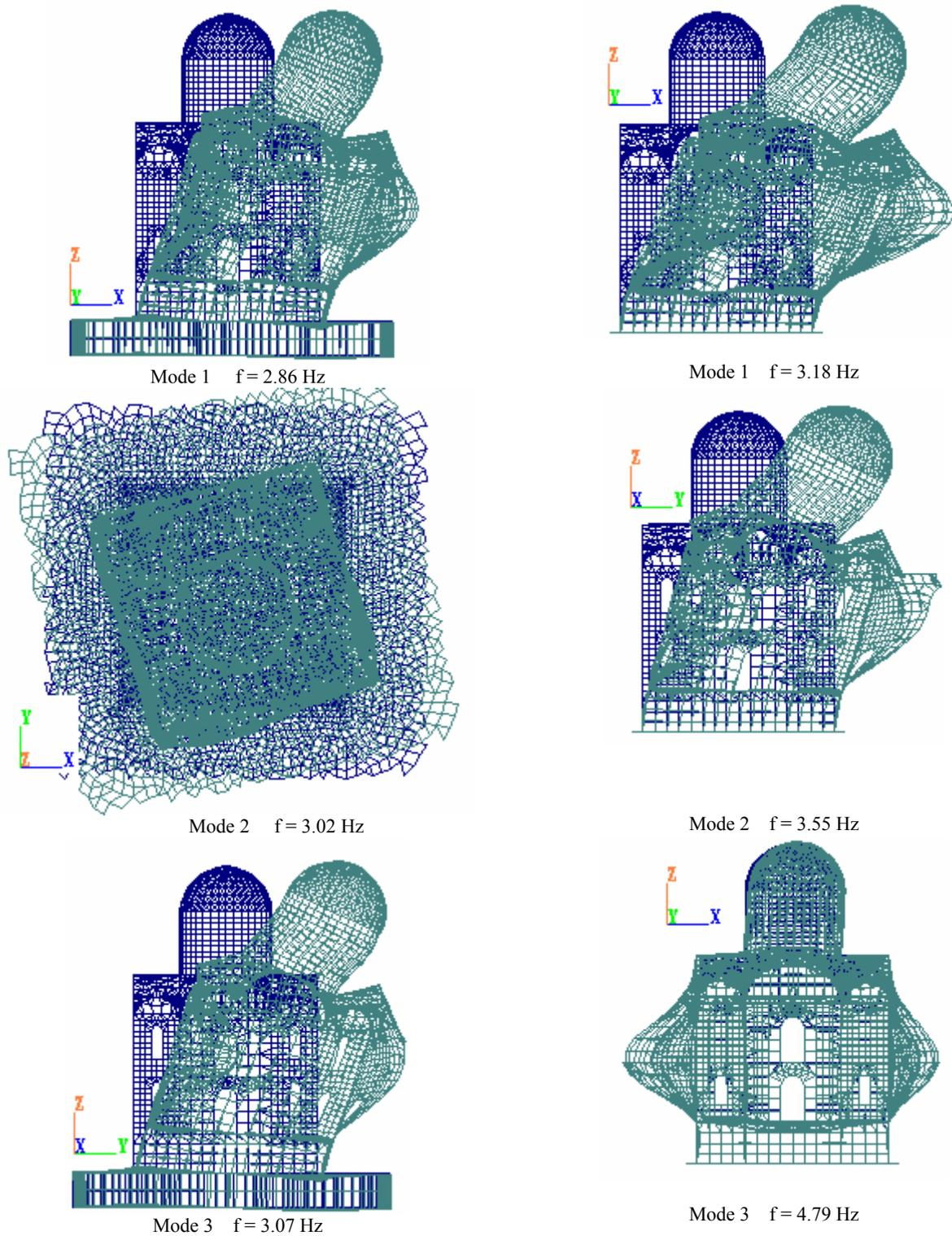
Fig 7 First three modes. A soil-structure system — on the left; a constrained structure — on the right
