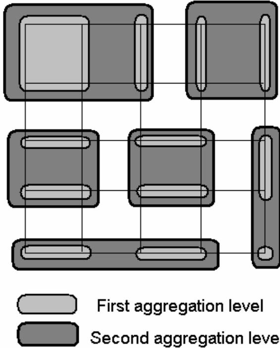
Fig.1 First and second aggregation levels for a rectangular plate with the finite element mesh 4x4
