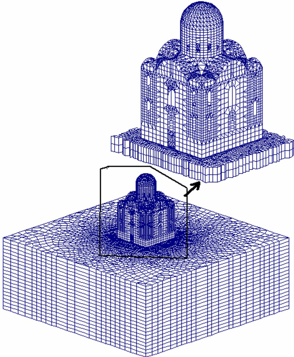
Fig.6 An example of a soil-structure interaction
